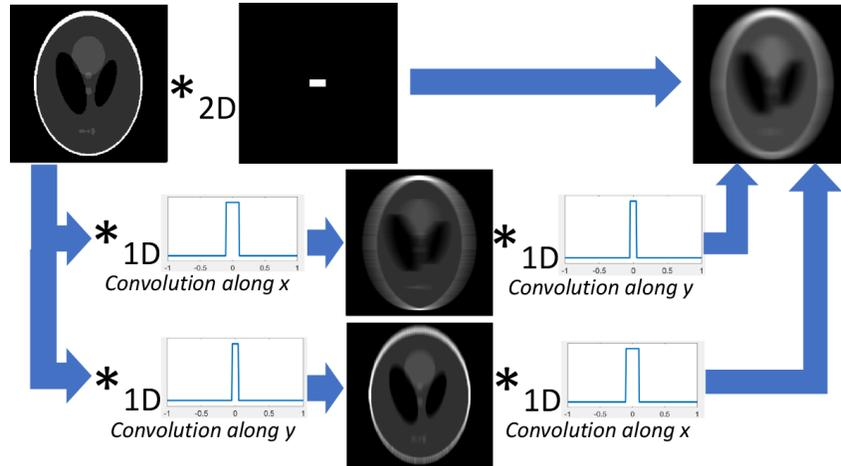
Figure 3.2: 2D convolution with a separable signal  $h(x, y) = h_1(x) \cdot h_2(y)$  can be done as two sequential 1D convolutions, with  $h_1(x)$  along  $x$ , and with  $h_2(y)$  along  $y$ , respectively.
